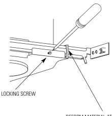
**DEFORM MATERIAL AT** ANY CORNER OF FRAME FOR ADDITIONAL LOCK IF NEEDED
